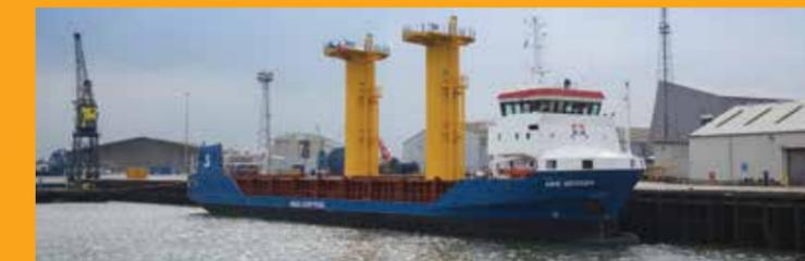
Each steel monopile is around 45m long and supports a 15m long transition piece, which includes all electrical cable connections.
